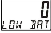
If battery charge is low, low battery message “Low Bat” will display. Please charge or change the battery.
