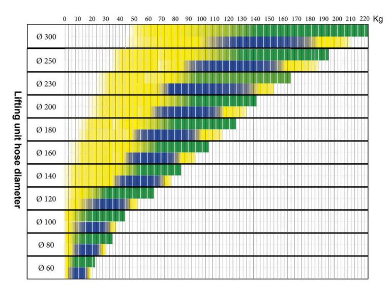
The bars in the chart show the recommended load weight for smooth, non-porous/porous material that can be handled by a specific lifting unit. combination. The recommendations are based on appropriate lifting speeds. Light loads are lifted more quickly than heavy loads. Solid material such as sheet-metal is lifted more quickly than porous material such as cardboard. Never use the lifting unit/pump combination for loads heavier than those recommended.
