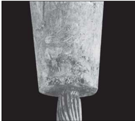
Typical example of the swelling of stainless steel rope due to crevice corrosion
