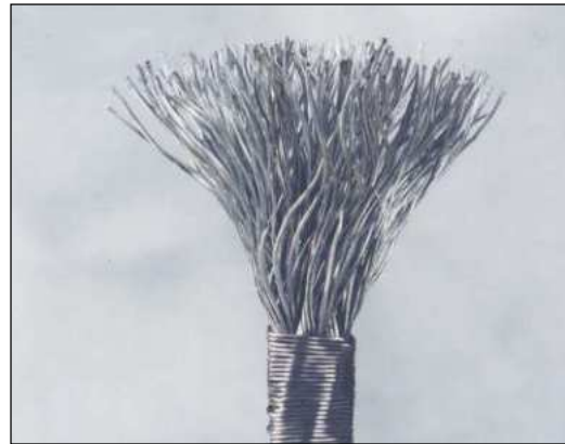
Properly Broomed Wire Rope (Fig. 2)
