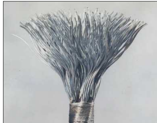
Incorrectly Broomed Wire Rope
