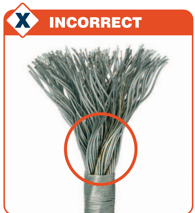
Figure 4: Incorrectly broomed wire rope.
