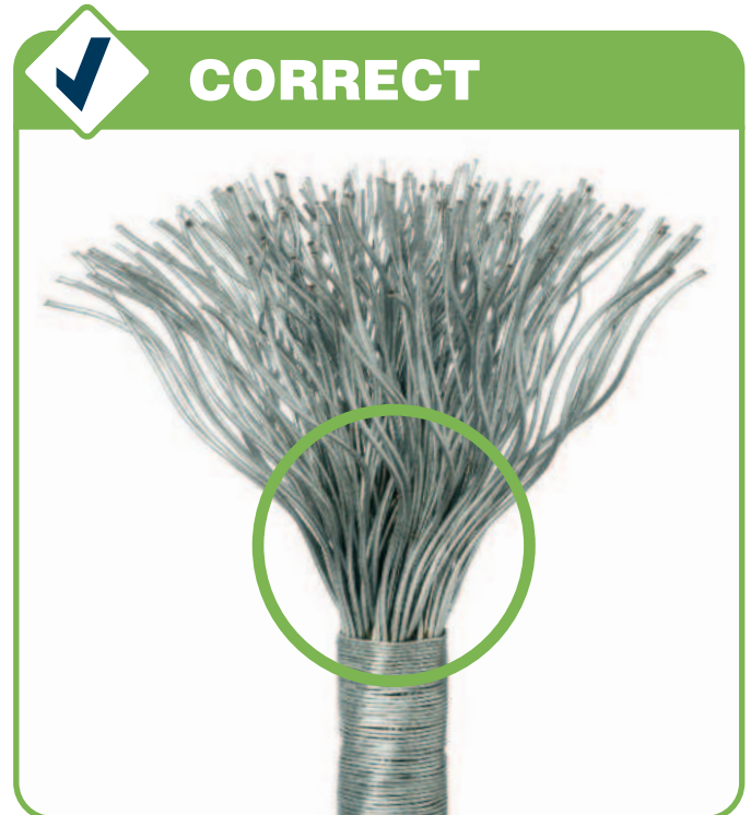
Figure 3: Properly broomed wire rope unlaid from the end of the rope to the seizing.
