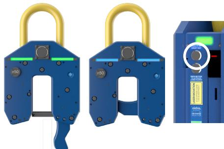
With the "Always On" mode, the colour code scheme of the LED status indicator will always be visible. Blue – for closed – and green – for open – are continuous for 10 seconds and then take an intermittent pattern in order to save battery. Activate this mode by pushing the top button beside the battery.
