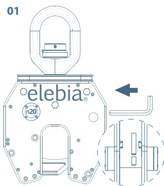
Insert 6mm hex key into slot/groove.
