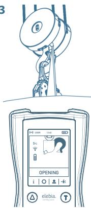
The NEO lifting hook unlocks and opens. (RED colour in LED status indicator. Do not lift)
