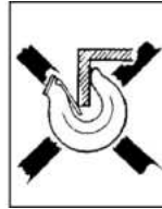
Fig 2 d Hook tip subject to additional bending stress
