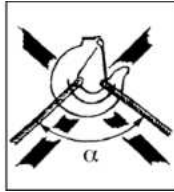
Fig 2 b Excessive top angle on sling! \alpha max 60°
