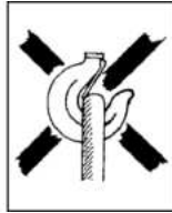
Fig 2 c Hook latch obstructed
