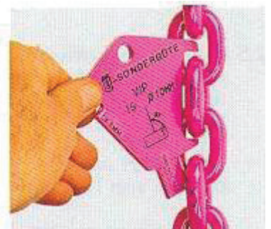
Testing plastic elongation caused by overloading
