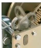
Reversible ratchet, 3 positions: up, down, free-wheeling
